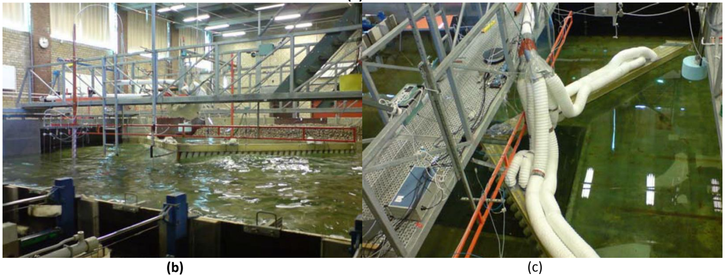
Figure 3-6: (a) LEANCON working principle and (b),(c) The LEANCON WEC 1:40 scale model in the deep 3-D wave basin at Department of Civil Engineering, Aalborg University (from [6]).
