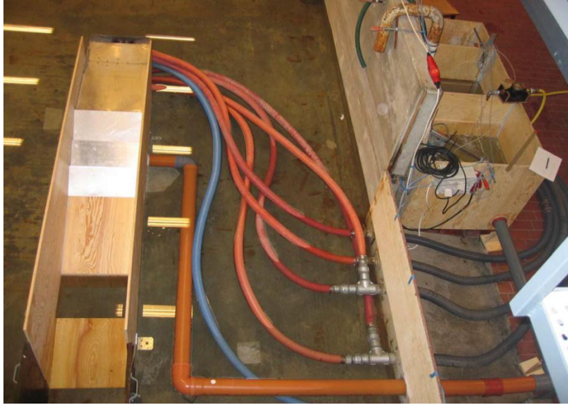
Figure 3-7: SSG overtopping device setup (from [7]).
